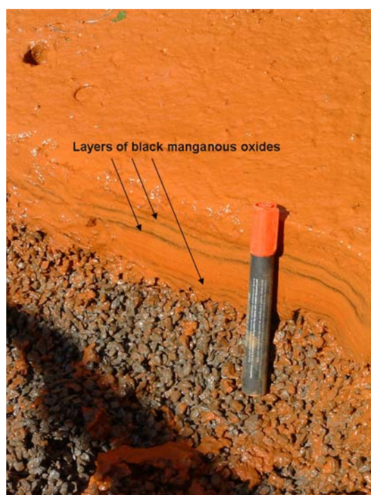
Fig. 3 Photograph of a cross-section of ochre sludge in the bottom of the VFR after decommissioning revealing layers of black manganous oxide
